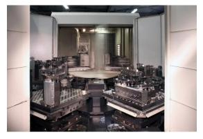
Mabotec's manifolds are getting more compact and the amount is increasingly becoming larger. Because of this, Mabotec had been looking for a clamping system which could be set up easily. Gressel MultiGrip's clamping systems were rapidly sought for as the solution.
